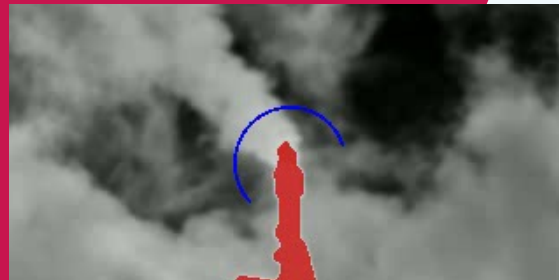
GP1 Survey Performed of 08/07/2022 Quantified Emissions: 2.078 mmscf/day
