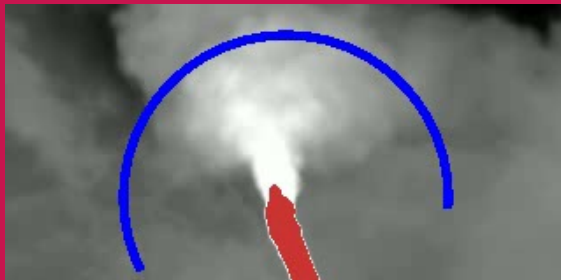
FC 37 Survey Performed of 06/07/2022 Quantified Emissions: 0.438 mmscf/day
